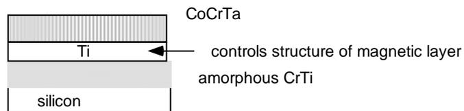
Figure D.4. Perpendicular recording using CoCrTa (Hitachi).
