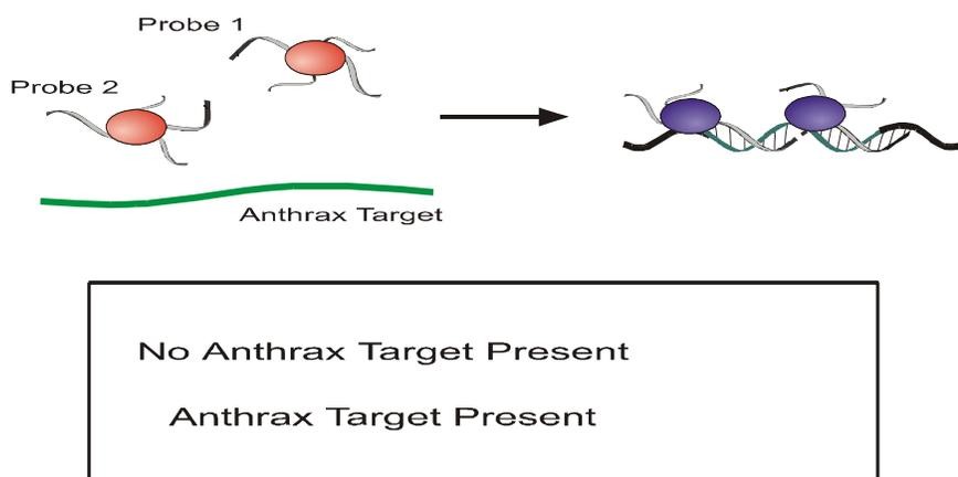
**Figure 8.8.** Anthrax detection: when the anthrax target is present, pairs of nanoparticles assemble together via the DNA filaments and change the color of the respective suspension (courtesy C. Mirkin, Northwestern University).
